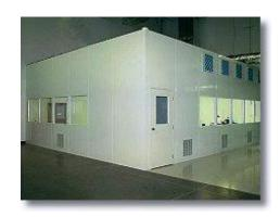
Doors are manufactured from the same wall panel material selected for the rest of the room. The perimeter of the door is reinforced and faced with aluminum channel. Unless specified otherwise, doors will have a paned viewing panel for safety, three spring closer hinge and lever passage hardware.
