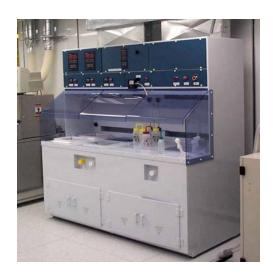
The use of polypropylene offers immunity to corrosion, resistance to acids and solvents, non-conductive properties, and a minimum of maintenance. Storage space is available underneath the work surface.
